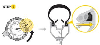
Turn to INFLATE mode then a strong blast of air will inflate the tire at the same time. If the installation is perfect, the bead of tire will snap into the rim as shown during inflation.
